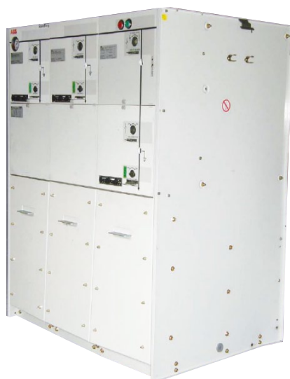
From IAC-test with arc suppressor
