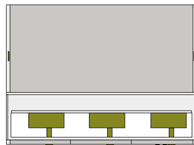
Top entry box seen from above when front/top covers have been removed.
